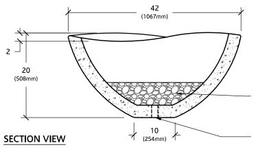
PLANTER MUST BE FILLED WITH MIN 6" CLEAR STONE AND FILTER CLOTH BELOW BEDDING SOIL
